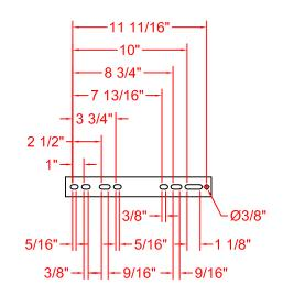
Note: Slide rails can be mounted on 8", 10-5/8", or 11-1/4" centers.
