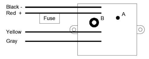
Connect the Black and Red wires to VDC power source (be sure to observe polarity noted). Make sure the amperage capacity of the power source meets or exceeds the requirements of the DC motor being operated with the unit.
