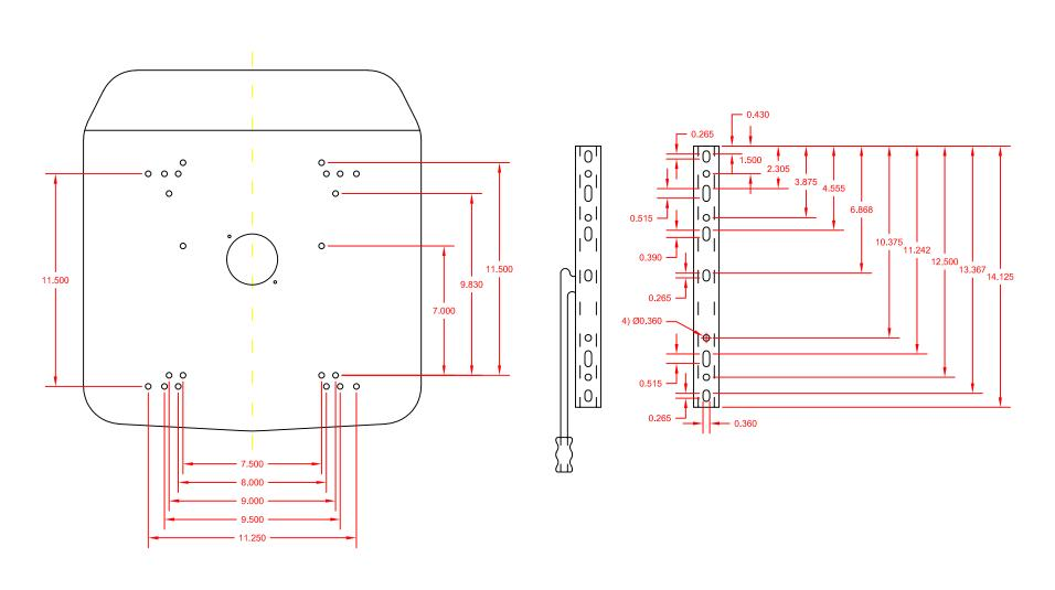
Some models of this seat are available with slide rails. Hole patterns in right and left slide rails match. Approximately 5.875" travel in slide adjustment.
