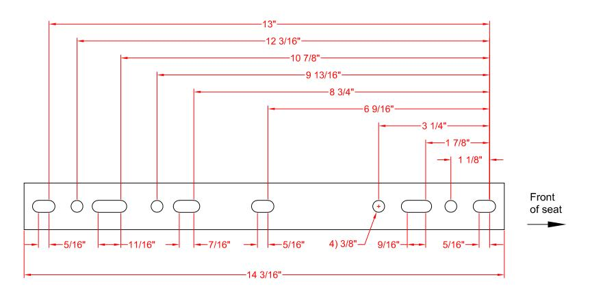
Left and right side slide rails have matching mounting holes Slide rails can be mounted on 11 1/4", 10 5/8", 8 3/16", 8", and 7 1/2" wide (side-to-side) spacings Approximately 5 7/8" travel in slide adjustment
